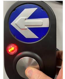
To test the Pendant Light (if fitted), push the button as shown.
