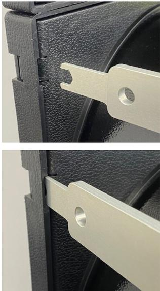
To gain access to the Light LED boards, use the custom tool provided by Data Signs.
