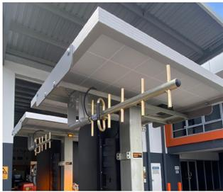
Each Traffic Light Trailer is fitted with a Directional antenna. This will provide reliable Wireless Radio (RF) communication between the PTL units; however, the units still need to be positioned line-of-sight to each other. The ends of each antenna should point *towards* the other. They can be adjusted on a swivel to help align the correct direction.
